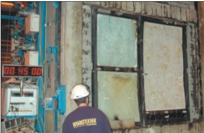
Test time 40 min, oven temperature approx. 900 °C
