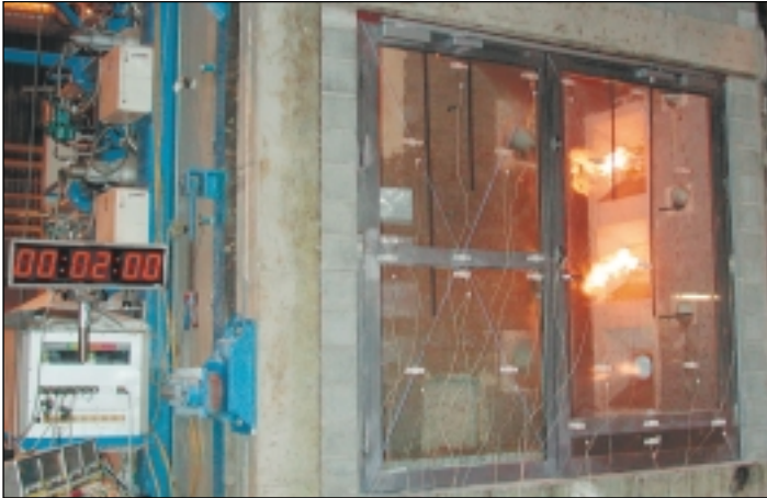
Test time 2 min, oven temperature approx. 300°C
