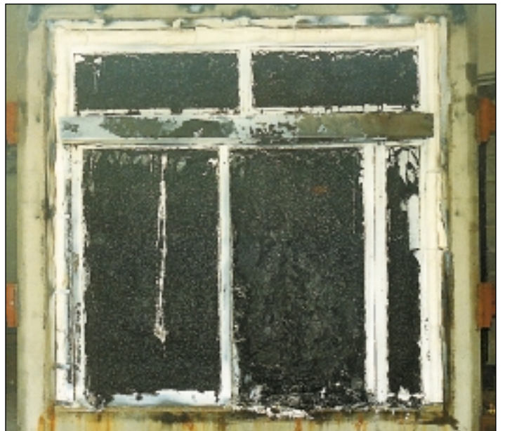
Sliding door fire test – exposed side after final testing 60 min
