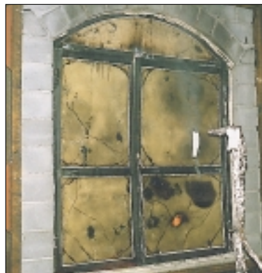
Fire test of door with finger trap proof gasket 60 min
