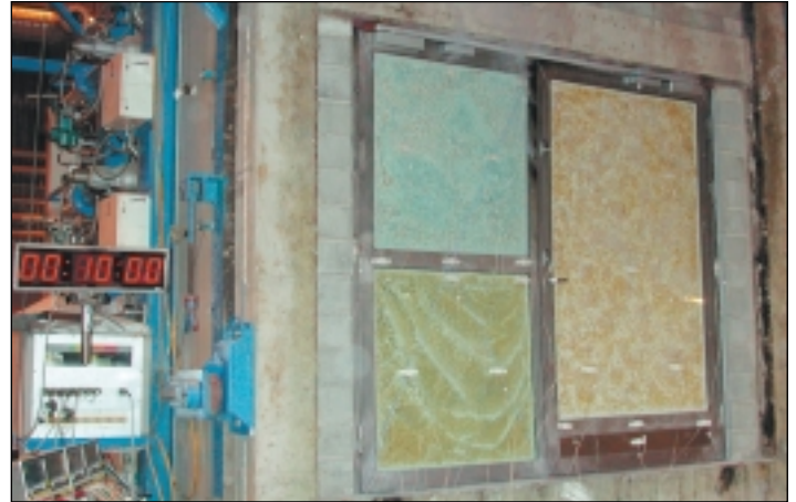
Test time 10 min, oven temperature approx. 700°C – deflection approximately 50mm
