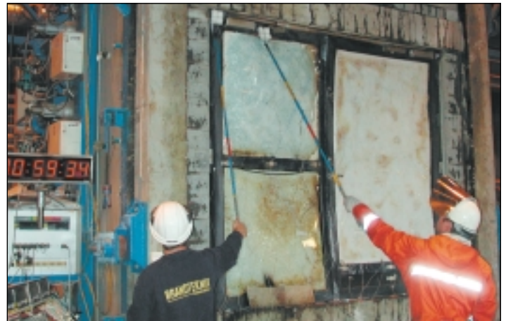
Test time 60 min – final control of the spread of fumes
