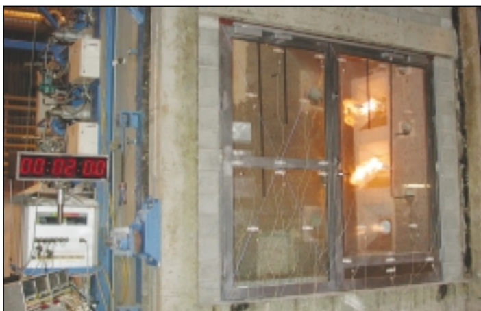
Testing time 2 minutes, oven temperature approx. 300°C
