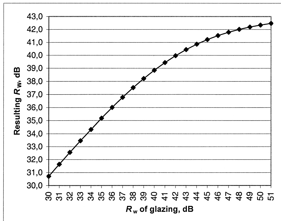
Figure 3 Resulting R_w of the complete facade as a function of R_w of the glazing unit s mounted in the facade. The steel profile has R_w = 36 dB, a value achieved by the profiles SP 56500/SP 956500 Door.
