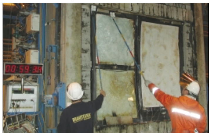
Testing time almost 60 minutes - final control of the spread of fumes
